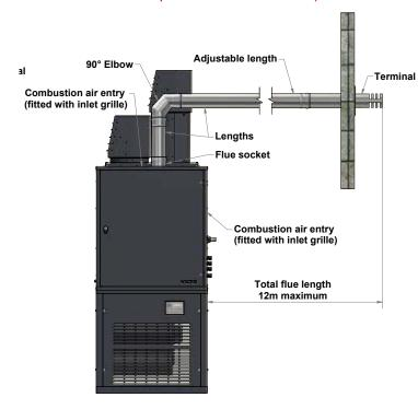
Flue Only- Vertical Flue System
