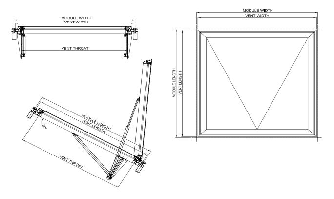
• Typical Vertical Ultrasky Detail (Bottom Hung - Chain Actuator)
