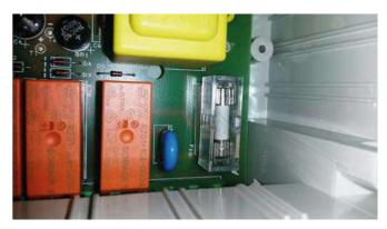
Isolate the power and remove the controller fascia pad. Pull off the clear plastic fuse cover and replace with new fuse.
