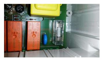
Isolate the power and remove the controller fascia pad. Pull off the clear plastic fuse cover and replace with new fuse.
