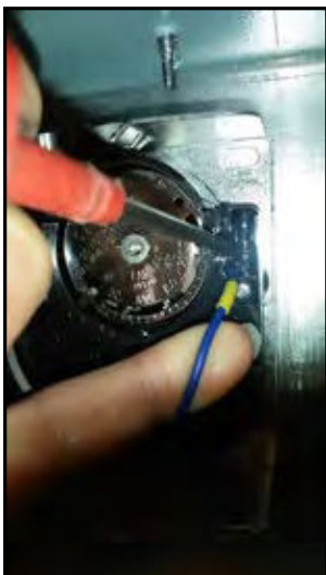
1.4 Remove all cables by pushing release catch then withdrawing the wire, noting cable colour connections.
