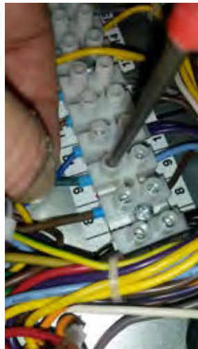
1.18 Replace brown live to t8 and blue neutral to t9 to terminal strip.
