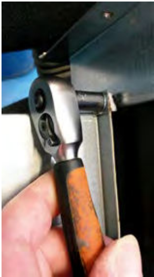
1.9 Remove fan outlet (if fitted) from fan.
